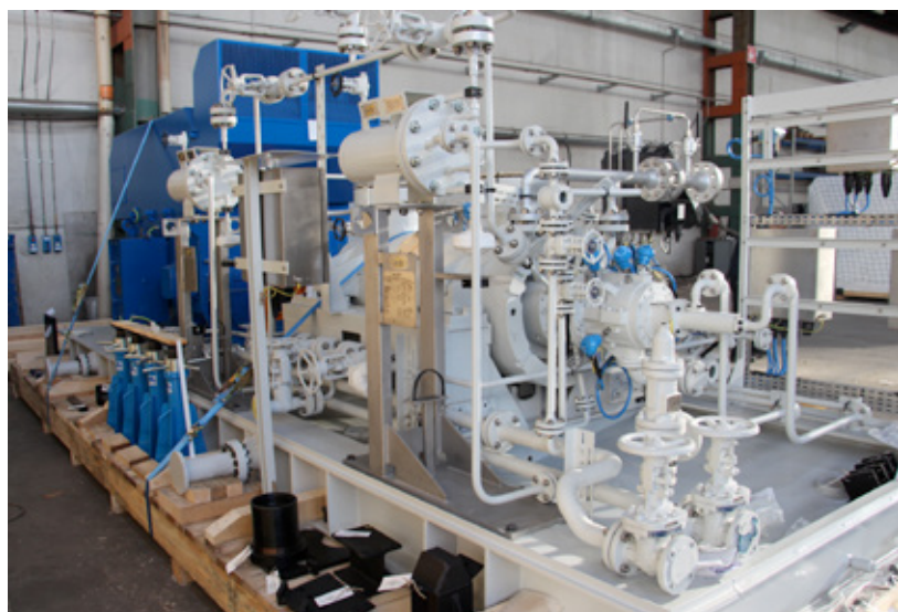
API 610 BB5-type HP boiler feed water pump for a petrochemical plant
