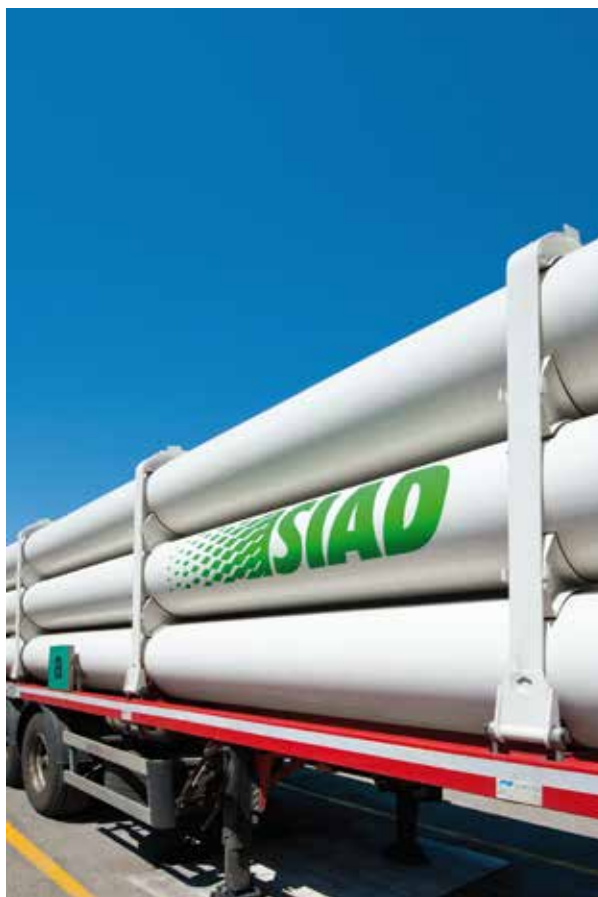
La flotta SIAD include carri bombolai da 200 a 500 bar (copyright SIAD)
