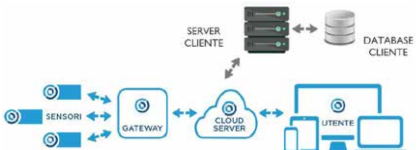
Fig. 7 - Cloud Platform: Real-Time data sharing
