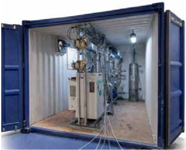
“Hymage” containerized pilot plant for e-methane and e-methanol production
