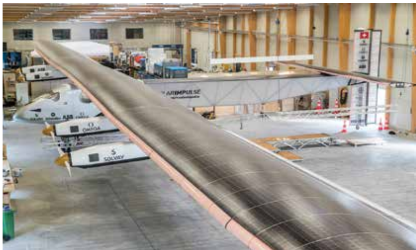
The microgrids installed on the wings of Solar Impulse
