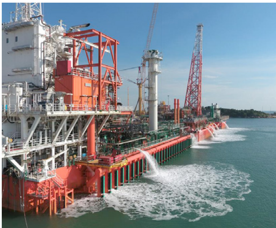
Ballasting during load-out
