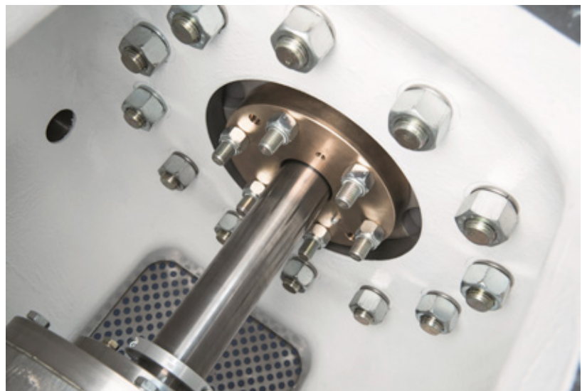
Picture 3: Oil free Design with Physical Atmospheric barrier
