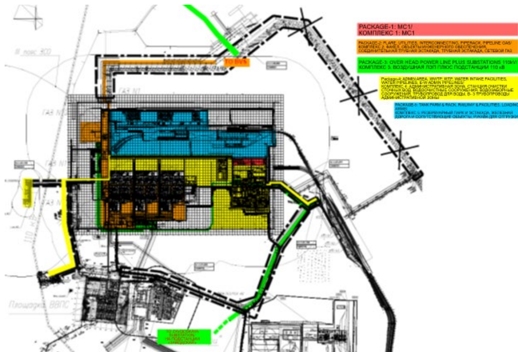
Figure 36 Example of Work Scope Subdivision in Work Packages
