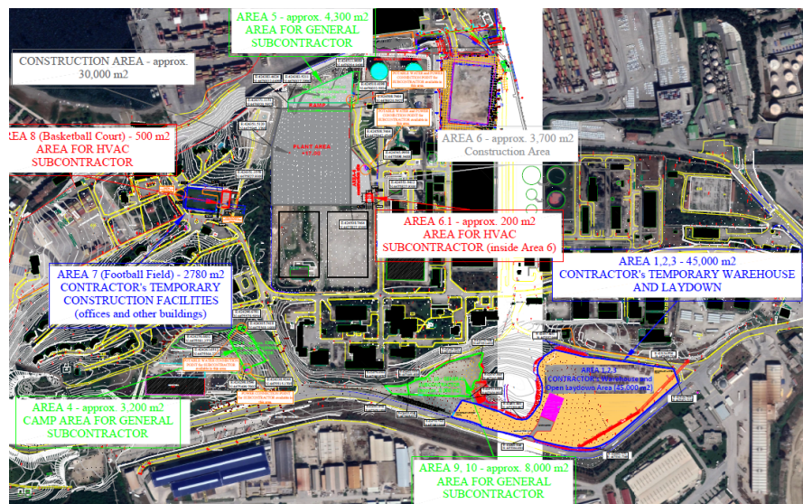
Figure 34 Temporary areas arrangement
